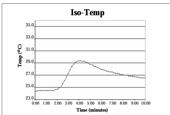
Figure 2c: Mean temperature of Iso-Temp during polymerization.
