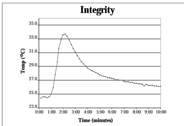
Figure 2b: Mean temperature of Integrity during polymerization.
