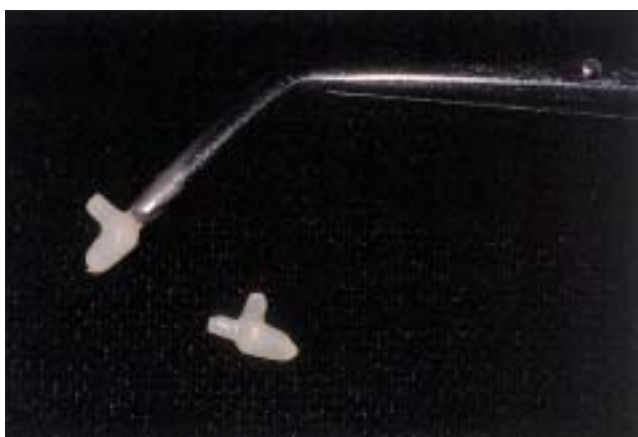
Figure 4: Beta Quartz glass-ceramic inserts, size L2, one held in a pair of tweezers.
