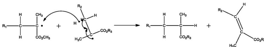
**Fig. 6 – For termination the polymerization process of methacrylates disproportionation is important. In this case, one molecule abstracts a hydrogen atom from the other molecule. This molecule forms a C=C double bond. The C=C double bond can be detected by Fourier transform infrared spectroscopy and leads to false low degree of conversion values.**
