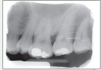
Figure 7: Storage phosphor sensor plate that is scratched and damaged at the edges.
