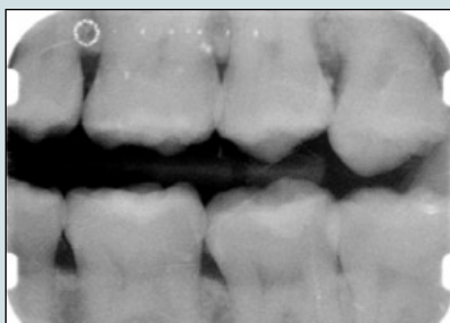
Figure 2: An image made on a photo-stimulatable phosphor (PSP) plate displaying widespread and severe damage to the PSP. This PSP should have been discarded long before it reached this state.
