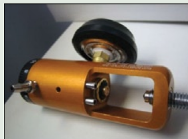
Figure 2: Regulator for an oxygen tank; note the presence of the washer.
