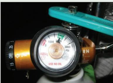
**Figure 1:** Pressure gauge for an oxygen tank showing 2000 psi.
