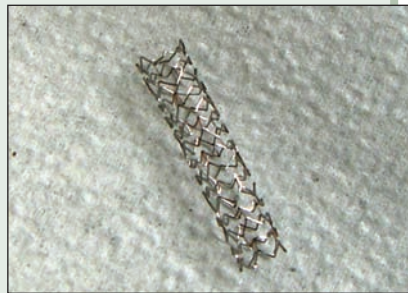
Figure 2: Coronary artery stent expanded as if it were inserted into the intima of the receiving vessel.
