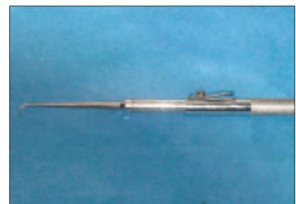
**Figure 3:** The spring-loaded back action hammer allows forces to be directed in a more controlled manner.
