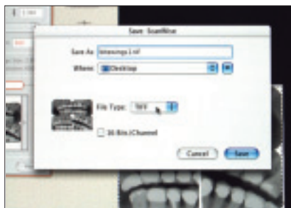
Figure 8: Create a “TIFF” file when you make your scan. Do not check the 16 Bits/Channel box, as this will create a needlessly large file.
