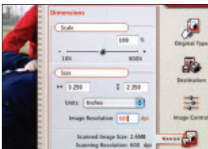
Figure 7: Scan at 500–600 dots per inch (dpi), at 100% scale.
