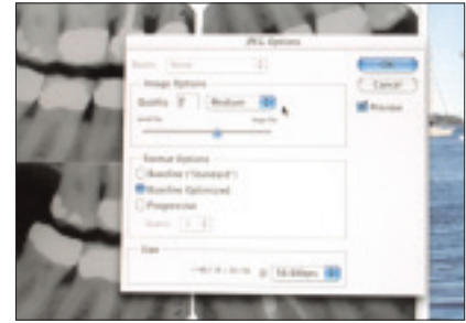
Figure 15: When creating a JPEG image, first try a “Medium” level of compression.
