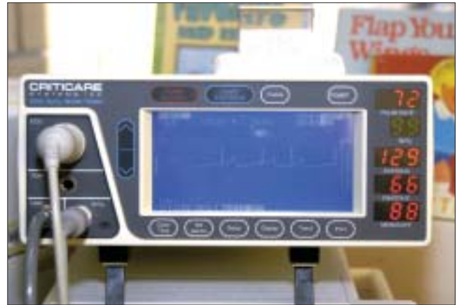
Figure 4: Appropriate monitoring is essential when sedating a child. This monitor measures heart rate, SpO 2 , diastolic and systolic blood pressure, respiratory rate and temperature, and provides a lead II electrocardiogram tracing.
