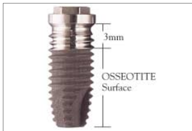
Figure 1: Osseotite implant: 3 mm polished coronal surface for soft tissue health and patented Osseotite acid-etched surface for increased mechanical interlocking with bone.
