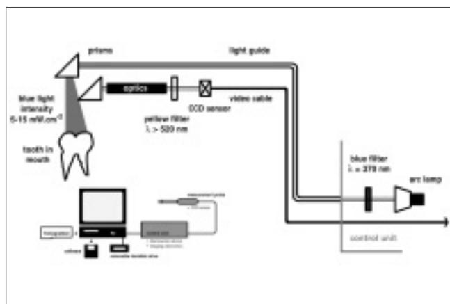
Figure 6: Diagrammatic representation of the QLF system.
