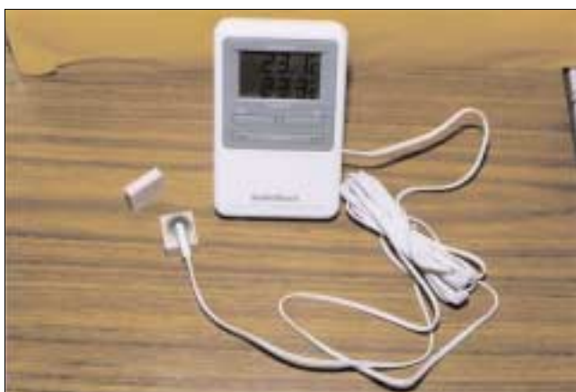
Figure 1: Mould and electronic thermometer used to measure temperature rise of resins.
