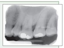
Figure 7: Storage phosphor sensor plate that is scratched and damaged at the edges.
