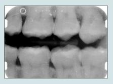
**Figure 2:** An image made on a photostimulatable phosphor (PSP) plate displaying widespread and severe damage to the PSP. This PSP should have been discarded long before it reached this state.
