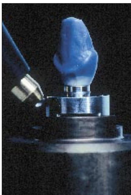
Figure 6: Verification of Procera abutment fit.
