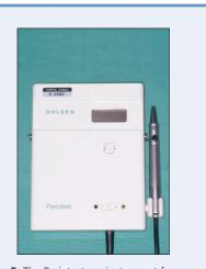
**Figure 5:** The Periotest: an instrument for quantification of tooth mobility that has been applied to the study of ankylosis. A low Periotest value, indicating less mobility, is not diagnostic for ankylosis. The reliability of this sophisticated device in this context is considerably less than the accuracy of the human ear in detecting ankylosis by simply tapping the tooth.
