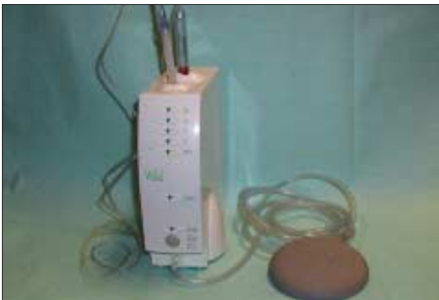
Figure 4: The Wand is a computer-controlled system consisting of pump unit, foot pedal, transfuser tubing, handpiece assembly, luer-lock needles and standard anesthetic cartridges.
